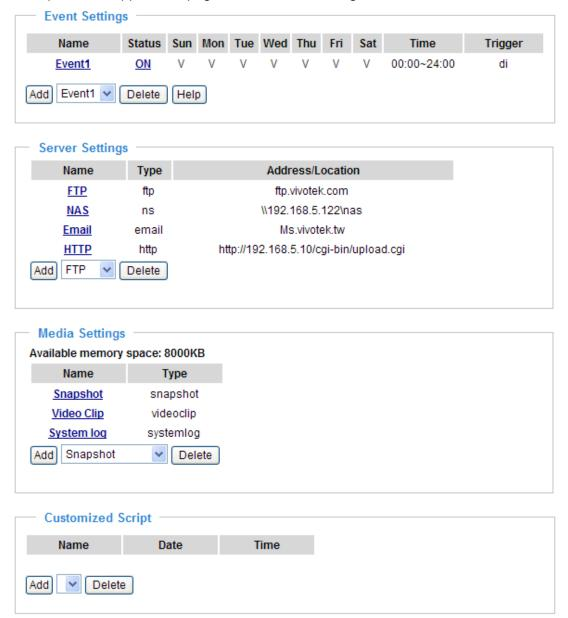
When the Event Status is **ON**, once an event is triggered by motion detection, the video server will automatically send snapshots via e-mail.
